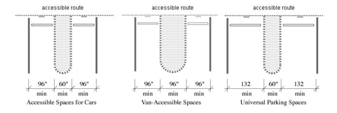
All three examples illustrated below show two accessible spaces with an accessible aisle and route.
