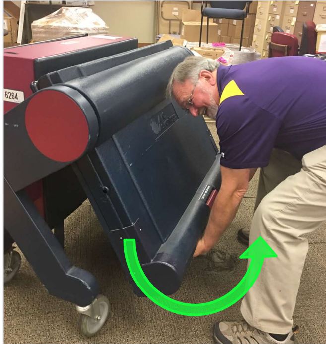
Figure 18: Positioning the Voter Panel to the Vertical Position (Part 1)
