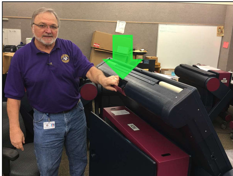
Figure 40: Maroon Latch on Voting Machine
