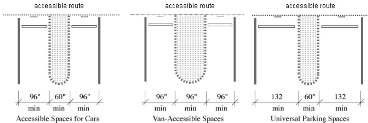
ii. The accessible parking and access aisle should be relatively level with no more than a 1:50 slope.
