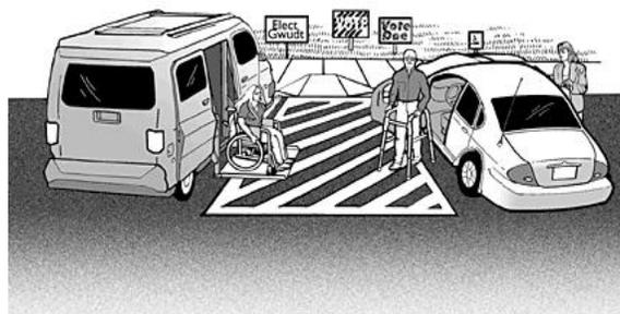
Notes for this illustration: Van-accessible parking spaces serve both cars and vans. A 96" access aisle is needed so a wheelchair lift may be lowered from the van onto the level surface.
